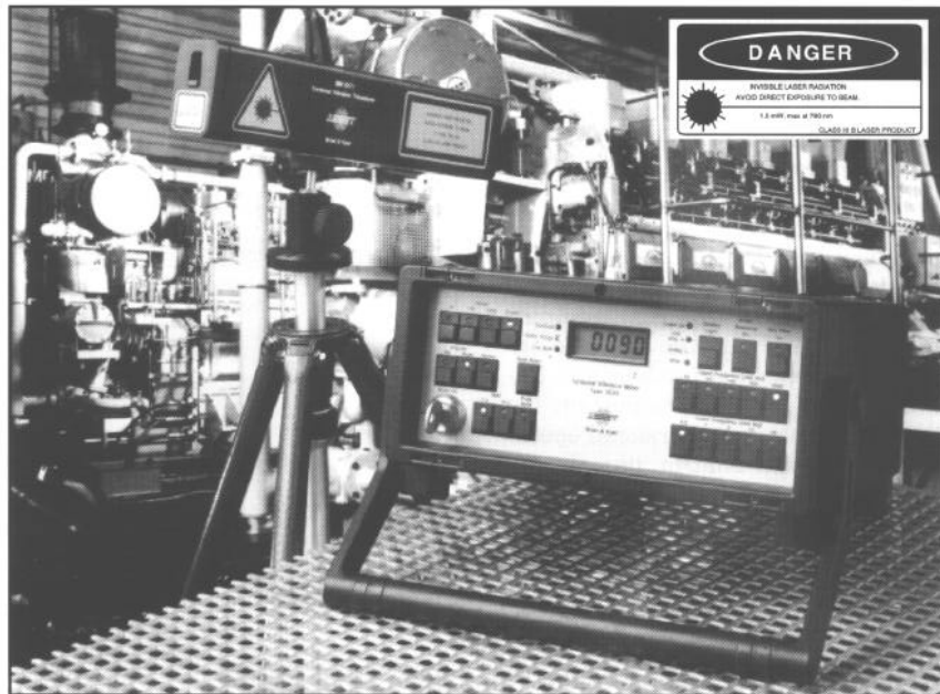
The Torsional Vibration Meter Type 2523 used in a TODS measurement
